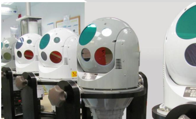
Multi-Spectral Gyro Stabilized Sensor
